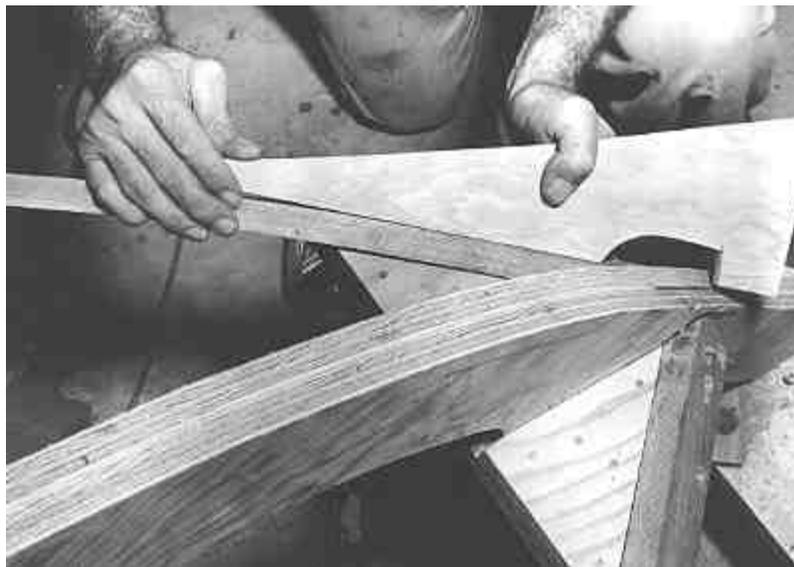
**T**he photo above illustrates a plywood fixture we have found helpful to determine the position of the chine on the stem side. Keep in mind what has been stated in the foregoing. The bottom and side must mate to the stem and chine on a continuous surface.
