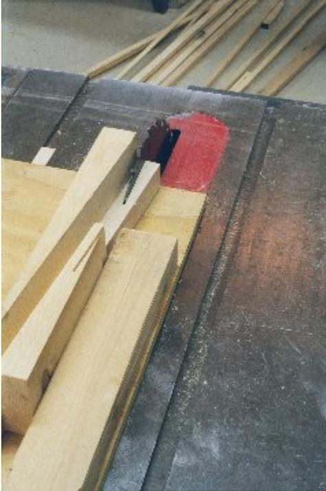
**H**ere the cut is shown in progress. Note the scars in the clamp wedge from previous cuts. You want to make sure that the saw goes completely through the batten so there is not a "nub" sticking out for later trimming by hand.
