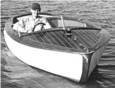
**C**utwaters were used on work boats to protect the bow and this carried through to stylish runabouts... chrome plated, of course. Some of the fancier cutwaters swooped back from about midpoint to the top to form a rearward facing arrow or other scroll ending. It was also common practice to cover the side at the transom ending with a chrome plated strip. These too often had a contour or curvature on the forward edge.
