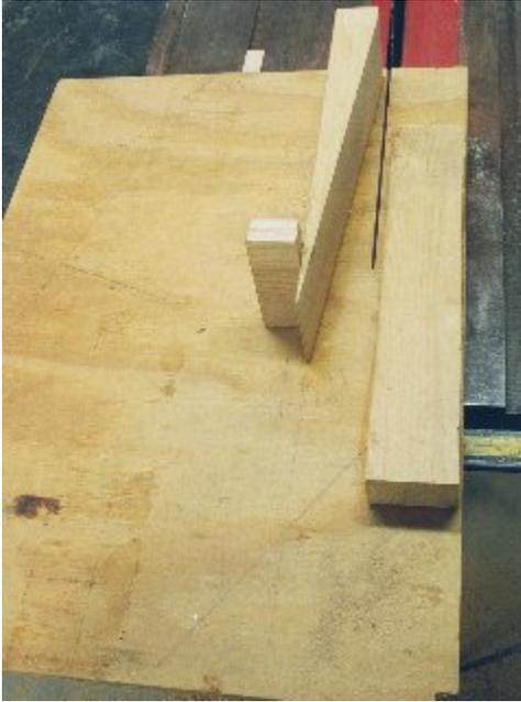
The angled fence and the wedge are from a 2x4 which had its edge jointed to square it up. The 2x4 was cut for an 8:1 slope as recommended in the plans. The wedge fence was glued and clamped while checking that it was absolutely square in the vertical direction.
