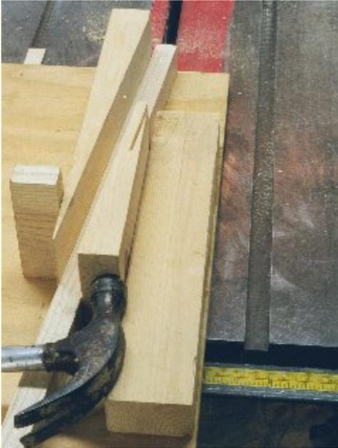
**C**hine piece ready for cut. The clamping wedge is shown being tapped into position with the hammer. The firm clamping is **VERY** important for repeatability.
